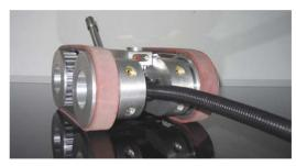
These Canadian-made robots are designed for difficult duct cleaning jobs.
