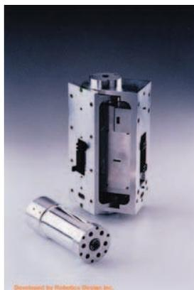
These modules are grouped together to form a stair-like shape, which handles a substantial load. The internal component holding the actuator of each module can be replaced, maximizing the applications and the functionality. This modular construction allows for manipulator configuration covering a broad range of sizes, payloads, and kinematics configurations for different applications, using all standard modules.
