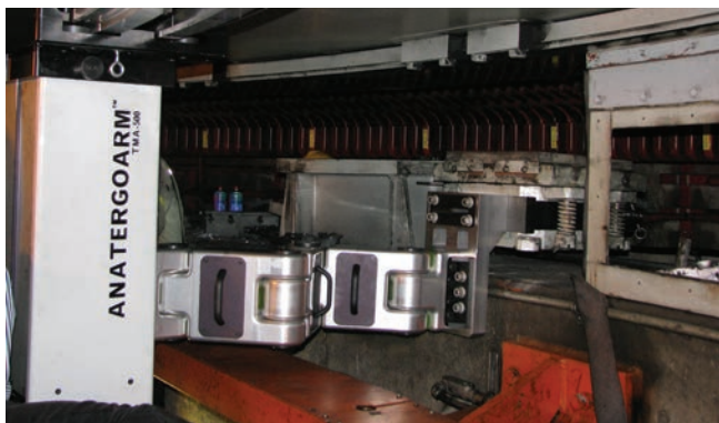
Like other ANATERGOARM models, the TMA-500 is composed of a series of H- and U-shaped modules that can support up to 500 kg.
