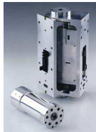
A compact portable version of the AMI-100, weighing 50kg, is able to manipulate 100kg with ease. Composed of a series of identical linked modules, the above prototype shows a robot with serpentine flexibility configured with 8-degrees of freedom.
