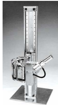
A compact portable version of the AMI-100, weighing 50kg, is able to manipulate 100kg with ease. Composed of a series of identical linked modules, the above prototype shows a robot with serpentine flexibility configured with 8-degrees of freedom.
