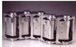
The robot's serpentine links arranged in a scara configuration increases robot flexibility and allows for maximum load capability.
